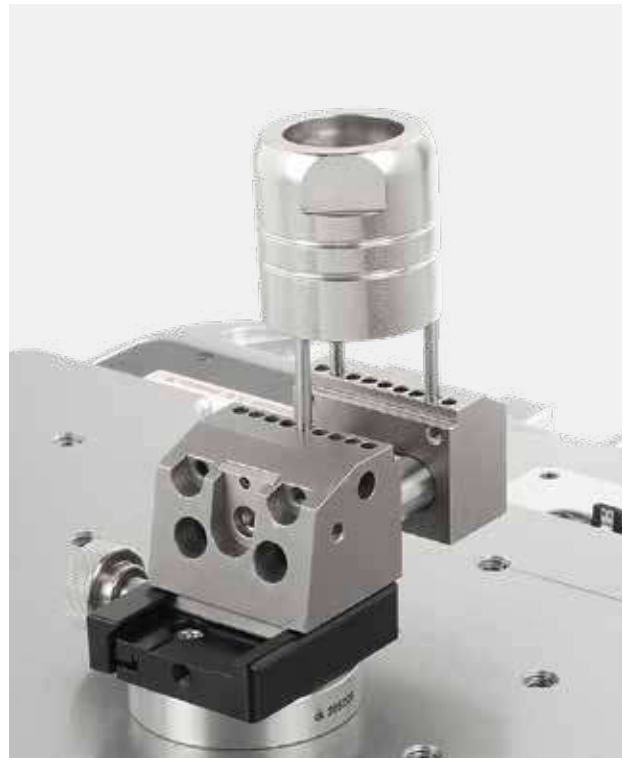
Internal clamping with pins for additional elevation.
